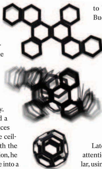
A series of photographs shows the transformation of a flat 4D-printed structure into a 3D object.
